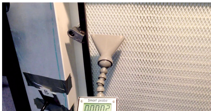
HEPA LEAK SCAN TEST
